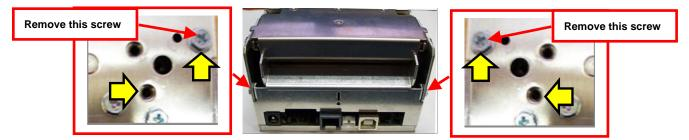
2. Remove the two Philip 3/16" Hex head screws on each side holds the back plate onto the printer. Do not remove the black plate.
