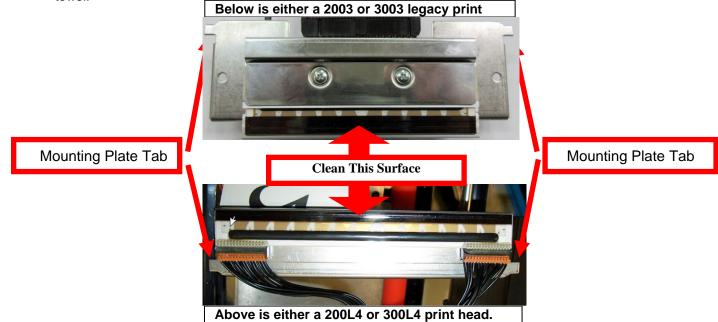
8. Install the head mounting plate by reversing the above procedures. Make sure the print head mounting plate tabs are in the correct print cage slots.
