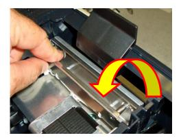
6. Lift the print head mounting plate straight out.
