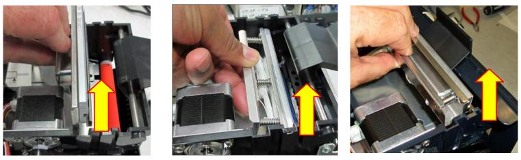
7. Clean the thermal print head surface (the side that makes contact with the paper) with isopropyl alcohol & paper towel.
