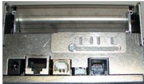
Above shows guide all the way to left for 3.22" wide media
