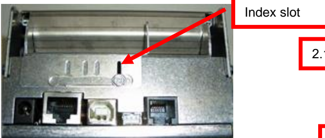
Above shows guide configured for 2.125" wide media
