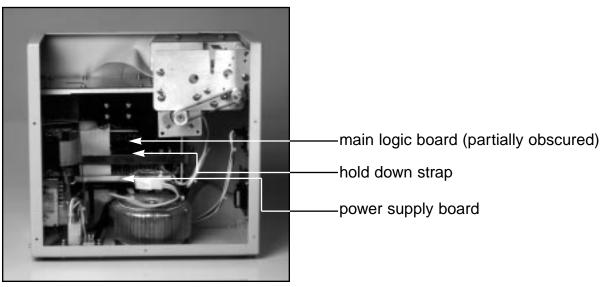
**Figure 5** - Vertical Micro - side view with electronics exposed
