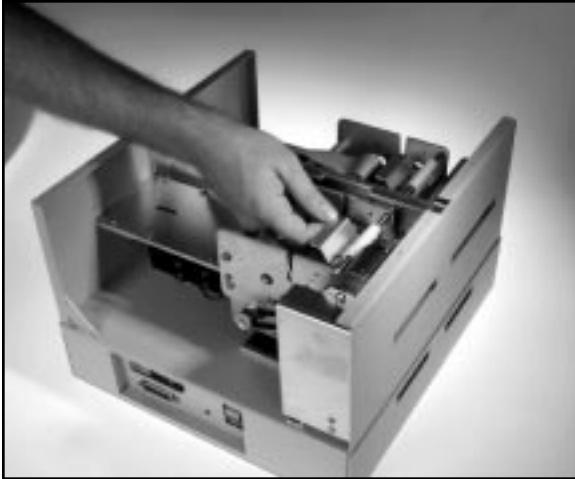
Figure 9A - Print Head removal
