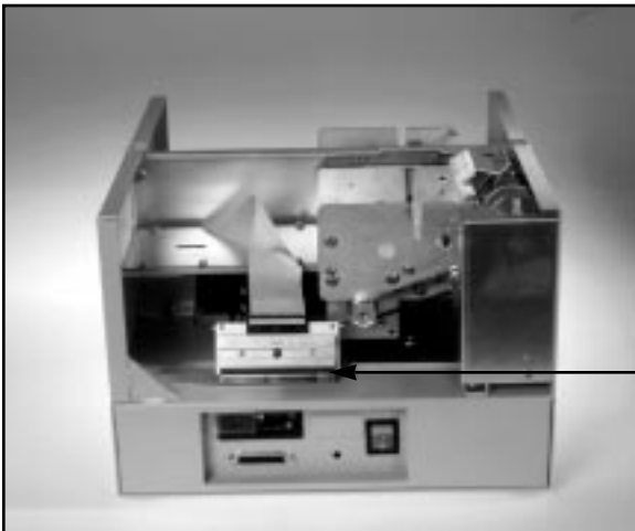
Figure 9C - Print Head removal
