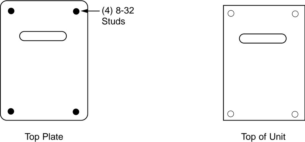
1. Attach Top Plate to Top of Unit so that studs protrude thru Top of Printer.
