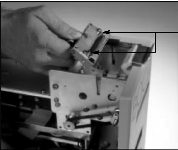
Remove these two unmarked screws to replace print head.
