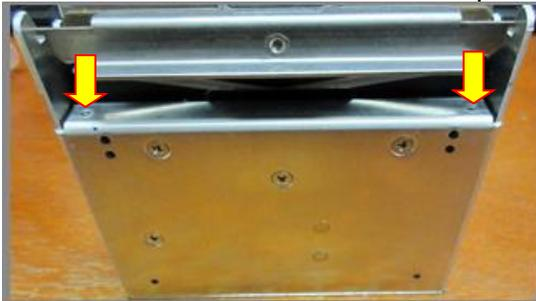
3. Unlock the print head assembly and lift up to allow easy access to the mounting holes.
