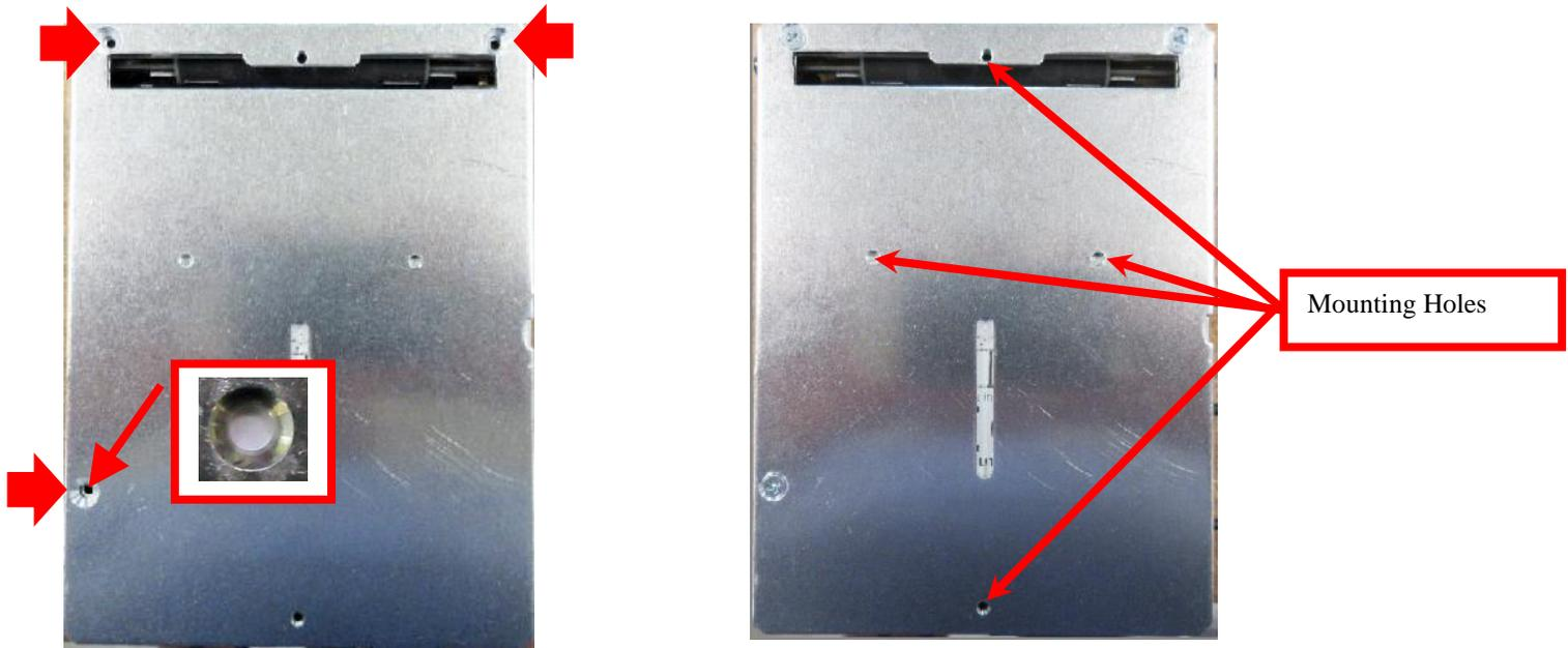
Care needs to be taken concerning mounting screw length, see guide below. ***The use of the incorrect length screw may damage the circuit board.***
