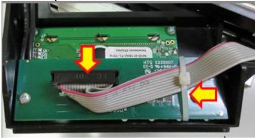
3. Plug the grey ribbon cable into the replacement control panel. Take care to make sure the keyed areas of the cable and connector line up.
