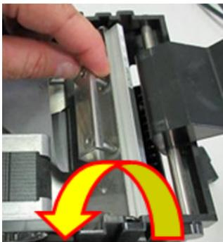
5. Lift the print head mounting plate straight out.
