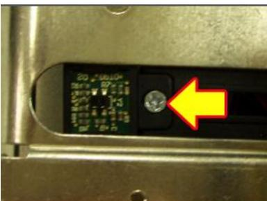
5. Plug the connector into the new replacement opto and install it back onto the mounting bracket.
