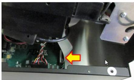
4. Denote where all the cables are plugged into the logic board. Gently unplug the cables from logic board.
