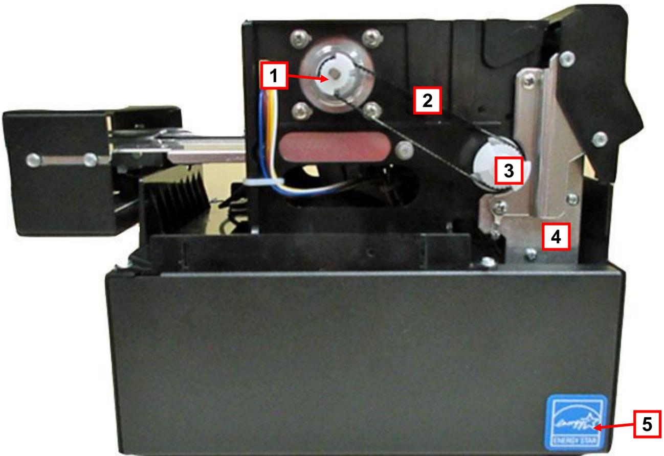
Above photo shows the Print Cage Pulley Cover removed
