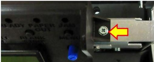
5. The electronics cover may be gently lifted up a little to enable the cutter assembly to separate from the print cage. This will enable you to get access to wires that connect to the cutter assembly. Cut the zip ties that hold the wires in place and unplug the wires. The cutter assembly can now be removed.
