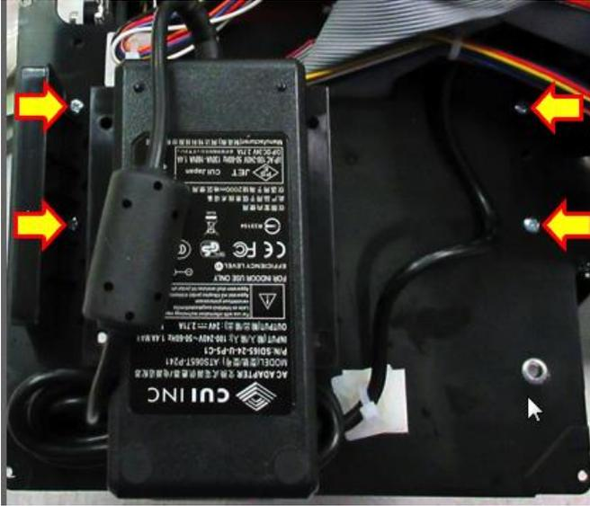
3. Once the screws have been removed the electrical cover may be gently tilted away from the print cage to gain access to the Load SQ Opto.
