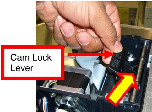
3. Position the cam lock level as far forward as possible.
