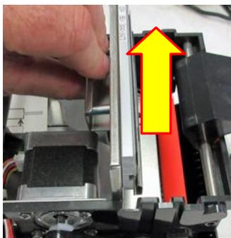
6. Clean the thermal print head surface (the side that makes contact with the paper) with isopropyl alcohol & paper towel.
