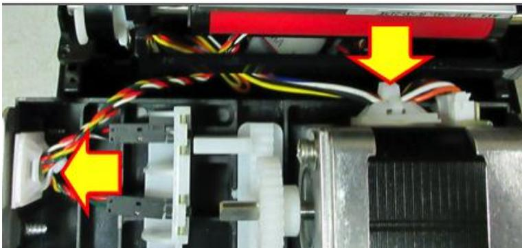
6. Connect the wires to the replacement cutter assembly and zip tie in place. Take care to make sure the wires are properly connected to their respective sensors. See photo below.
