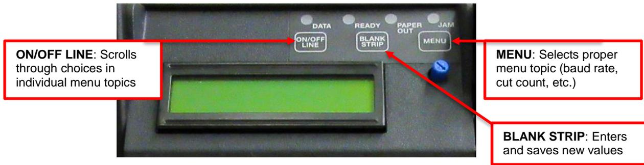
The printer has four LED lights on the control panel. All LEDs will illuminate briefly after power up.
