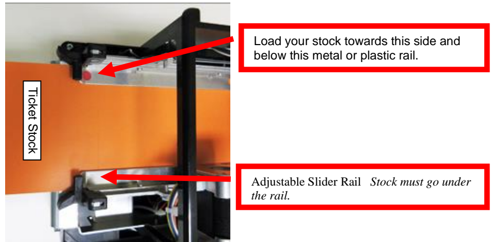
Above photo is of RADJW UPG with metal rails paper path set for 3.25" wide stock
