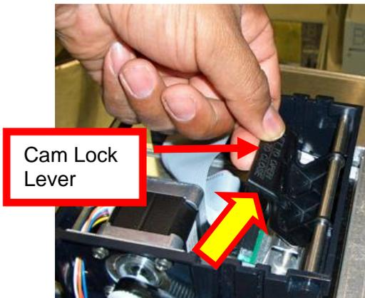
4. Position the cam lock level as far forward as possible.
