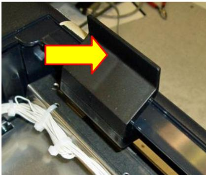
5. Flip the head back toward the rear of the printer. Denote what slot the print head was taken out of. Below photos show the different type of head mounting plates used through the production history of the Lemur series printers.
