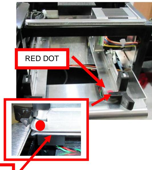
Blow air in this area. Between the upper and lower rails
