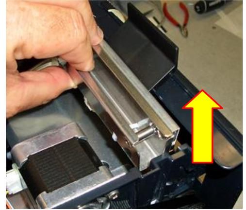
7. Clean the thermal print head surface (the side that makes contact with the paper) with isopropyl alcohol & paper towel.
