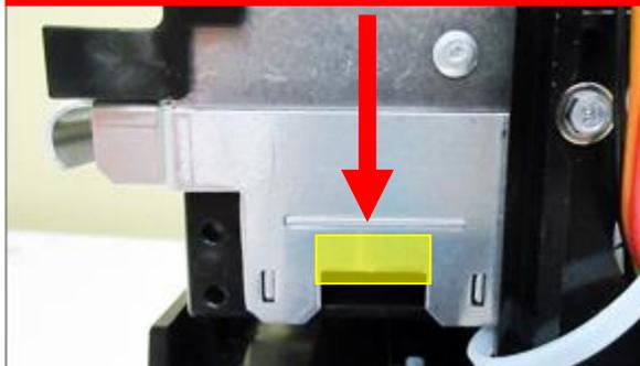
The adjustable rail may be opened by gently pushing on the paper guide rail (highlighted in yellow) with your thumb.
