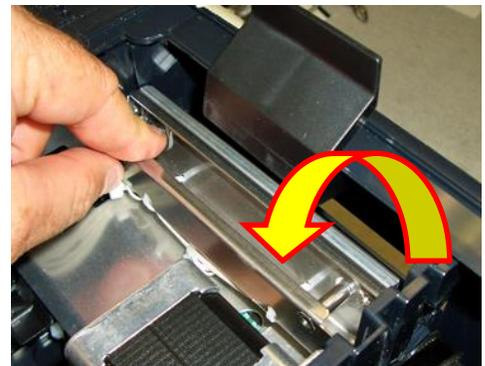
6. Lift the print head mounting plate straight out.
