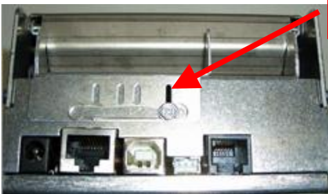
Above shows guide configured for 2.125" wide media
