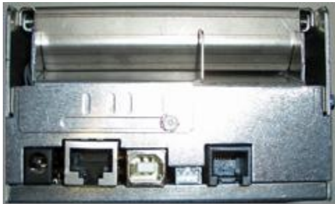
Above shows guide all the way to right for 2" wide media
