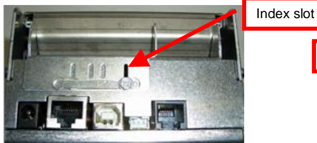
Above shows guide configured for 2.125" wide media
