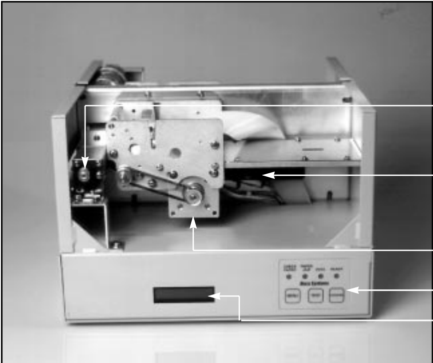
Figure 2a - Dual Mini ticket printer (LCD/Control Panel)
