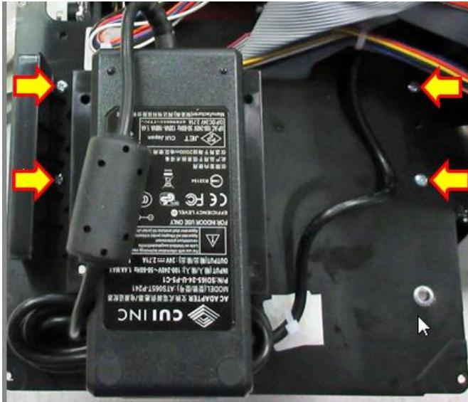
4. Once the screws have been removed the electrical cover may be gently tilted away from the print cage to gain access to the SQ load opto.
