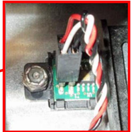
5. Remove the 1/4" nut with either a nut driver or socket.
