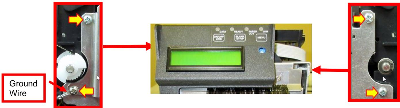
go on the same side the ground wire and pulley are on.
