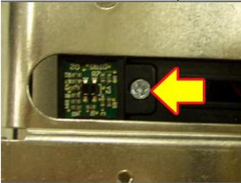
5. Plug the connector into the new replacement opto and install it back onto the mounting bracket.
