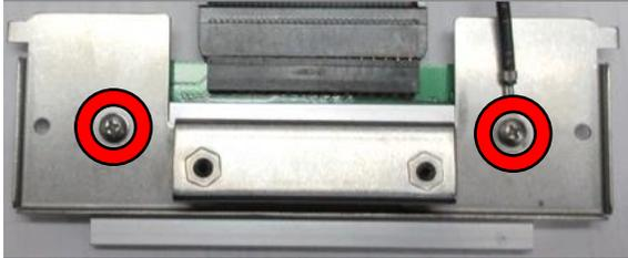
3. Gently unplug the cable from the old print head and plug it into the new print head. If your print head has two cables then this should be done one cable at a time so not to mix them up. The cables are keyed (see examples below). The keyed position must be lined up while plugging the cable into the print head. **You should not have to use excessive force to do this.**
