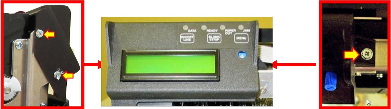
3. Remove the Philip head screw that secures the ground wires to the cutter assembly.
