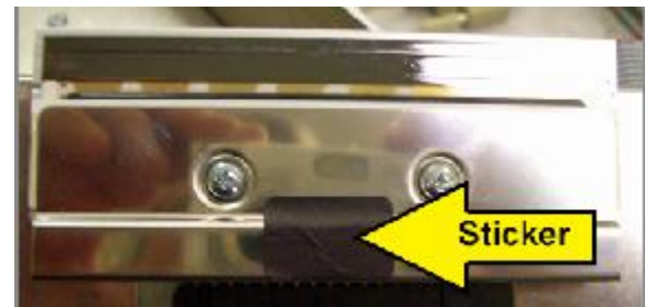
Above photo is of a Lemur-M built after February-2015 that has a SQ load opto. S/N 320833 & higher. This type of printer requires a black sticker to be on the bottom of the print out over the SQ opto location. See photo below.
