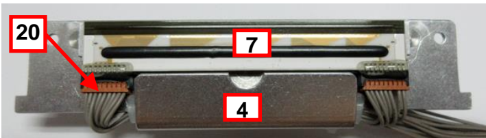
200C3 print head installed on 423496-ONE2C head mtg. plate
