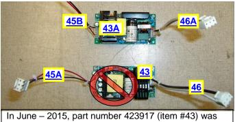
phased out for 424031 (item #43A). If installing a 424031 power supply in place of a 423917 power supply you will need to order associated cables too
