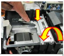
Pushing down on the head cable will aid in flipping the head plate.
