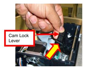
4. Position the cam lock lever as far forward as possible.
