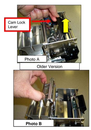
In January of 2017 was phased in the use of spring tension head mounting plates (s/n 378067 and higher). Below reviews how to remove this type of head mounting plate.
