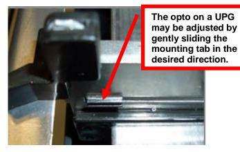
Note: Before making any opto adjustments make sure your ticket stock was manufactured to proper <u>ticket</u> <u>specifications</u>.
