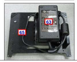
Lemur & Lemur-K printers built after below dates used a 424009-L power pack: June-2016 <u>220VAC</u> S/N 366455 & higher August-2016 <u>110VAC</u> S/N 371579 & higher
