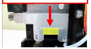
The adjustable rail may be opened by gently pushing on the paper guide rail (highlighted in yellow) with your thumb.
