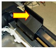
5. Flip the head back toward the rear of the printer. Denote what slot the print head was taken out of. Below photos show the different types of head mounting plates used through the production history of the Lemur series printers.
