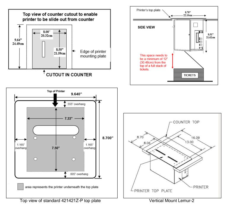
If you are looking to make the cutout just big enough to fit the printer then we recommend making the cutout 0.50" larger than the height and width of the printer.
