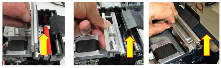
7. Clean the thermal print head surface (the side that makes contact with the paper) with isopropyl alcohol & paper towel.
