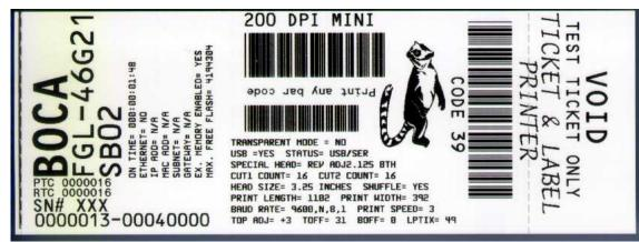
Above sample was printed on a 2" x 5.5" ticket using a 200dpi FGL protocol Lemur with cutter.
