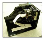
Above photo is of a plastic cabinet Lemur-S with optional cutter and cover removed. Your printer may vary. Two typical ticket formats and feed directions are shown below. The black timing mark must be facing the opto sensor.
