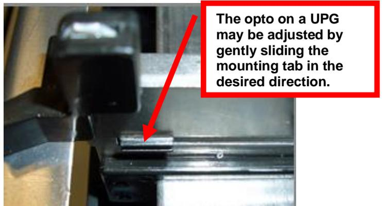
Note: Before making any opto adjustments make sure your ticket stock was manufactured to proper [ticket specifications](#).
