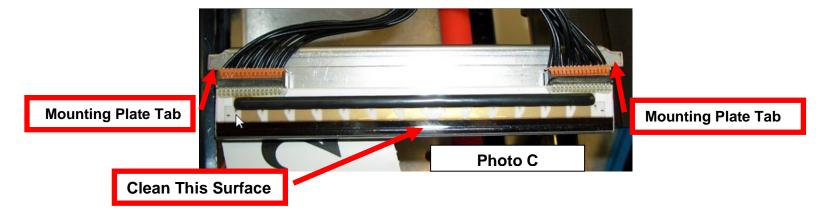
When install spring tension head mounting plate black in place make sure the mounting plate tabs are both aligned with the front slots (see below photos).
