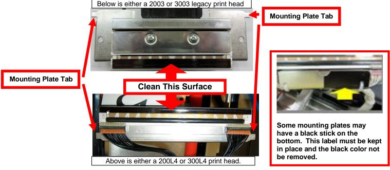
8. Install the head mounting plate by reversing the above procedures. Make sure the print head mounting plate tabs are in the correct print cage slots.
