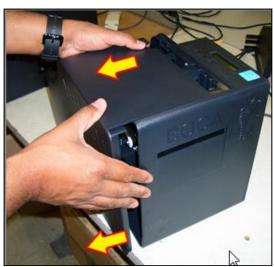
While holding down the locking tab, slide the cover outward towards you.
