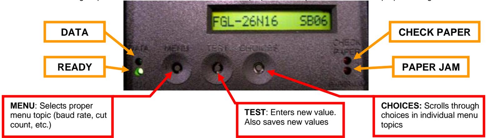
The printer has four led lights on the control panel. All led will illuminate briefly after power up.
