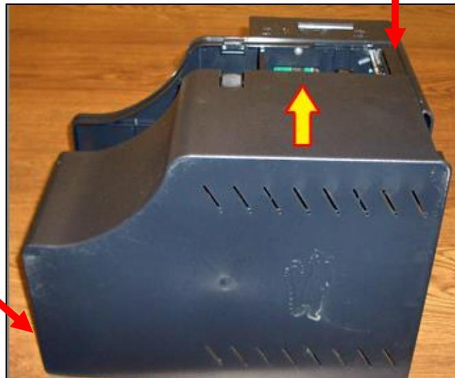
The cover may be installed by reversing the above procedure. Once you align the top and bottom part of the cover with the cabinet, slide the cover away from you until the tab locks.
