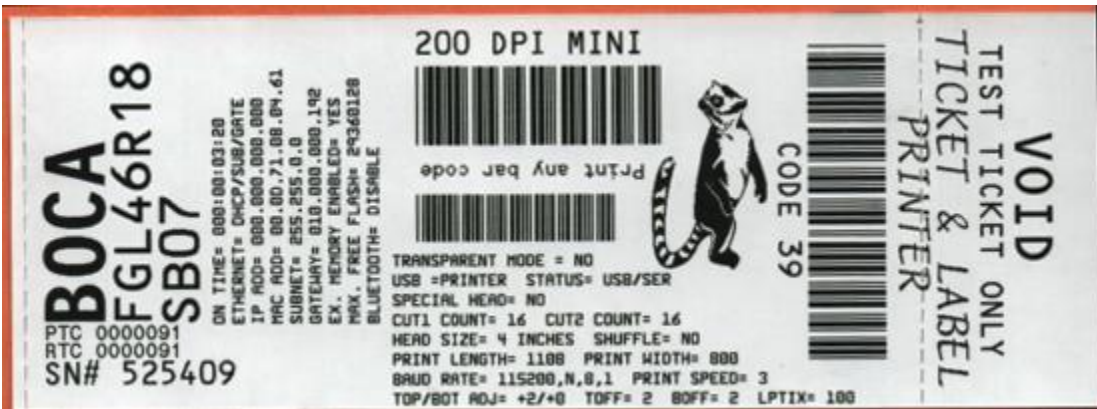
Above sample was printed on a 2" x 5.5" ticket using a 200dpi FGL protocol printer.
