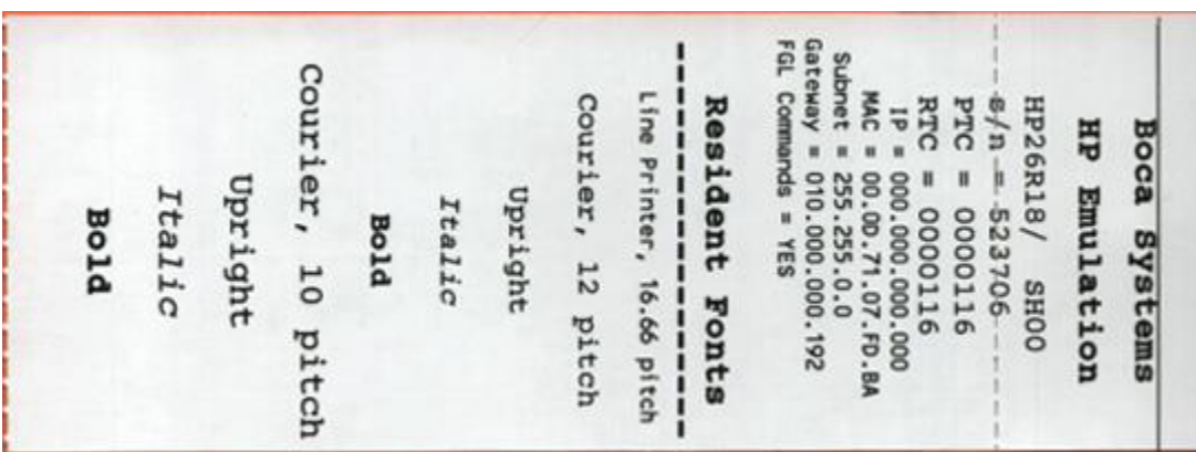
Above sample was printed on a 2" x 5.5" ticket using a 300dpi PCL protocol printer.
