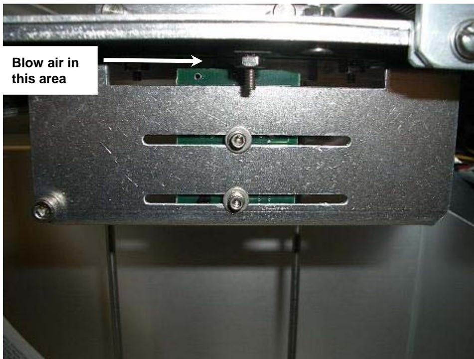
There is one opto devices mounted on a silver aluminum bracket beneath the paper guide. The opto controls ticket cut/tear position. Over a period of time there may be an accumulation of ticket dust on the opto eyes themselves. This paper dust could cause erratic operation of the printer.
