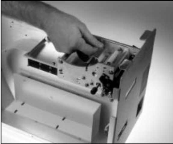
Figure 8A - Print Head removal
