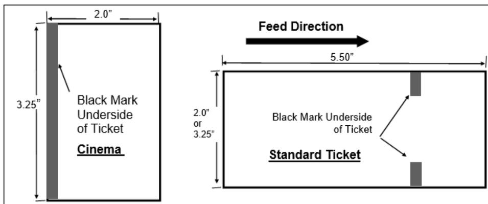
When loading 5.50" long ticket stock the black timing mark should be closest to the leading edge of the ticket (the first part that goes into the printer). When loading 2.0" long cinema ticket stock the black timing mark should be furthest away from the leading edge of the ticket (the first part that goes into the printer).
